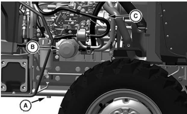
A—Oil Drain Plug B—Oil Filter C—Oil Fill Cap
