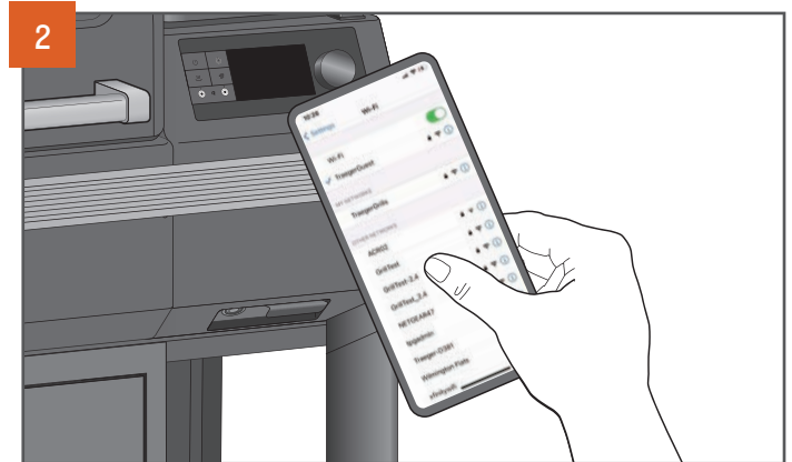
2 Ensure your smart device is connected to the Wi-Fi network to which you want your grill connected. The router signal must be 2.4 GHz.
