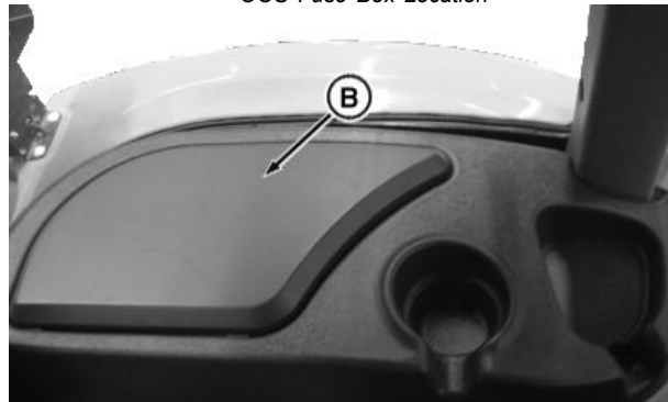
Cab Fuse Box Location
